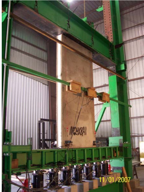
Figure 3A: Front view of wall and instrumentation setup
