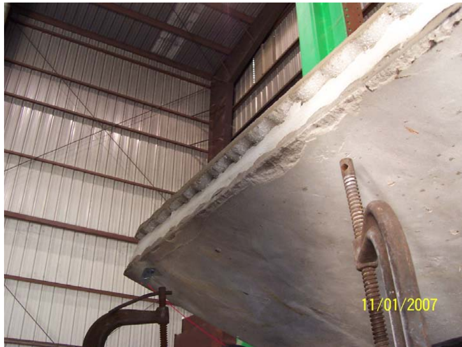
Figure 6A: 4X8A1 Failure mode (close-up at top)
