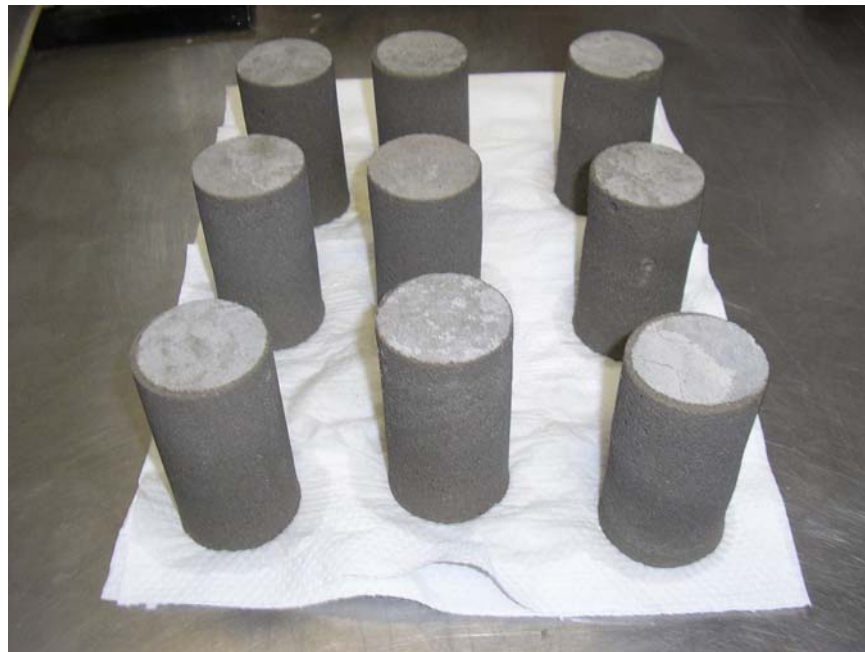
Figure 18: Mortar cores after drilling
