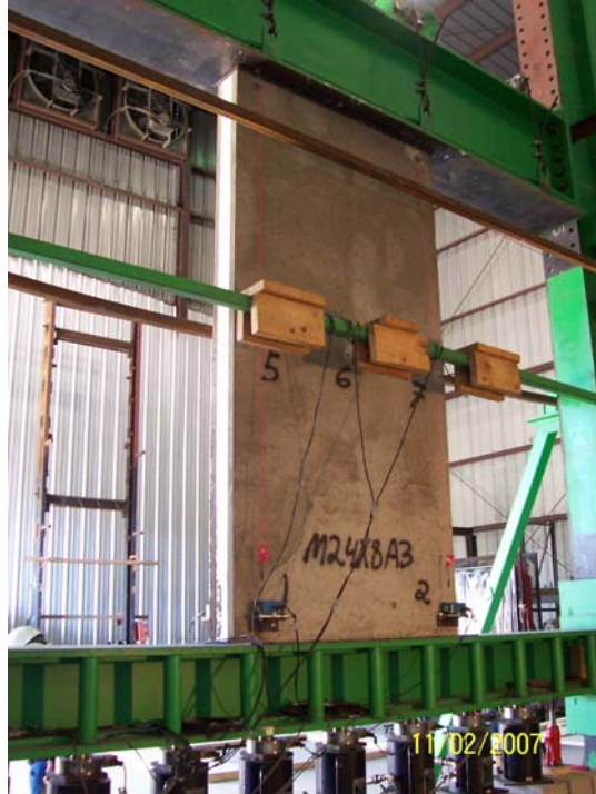
Figure 8: Axial test setup for 4' x 8' walls (overall view)
