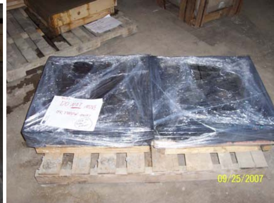
Figures 15 and 16: Mortar form labeling and sealing with plastic sheathing
