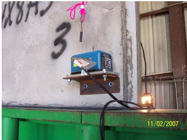
Figure 9: Axial deformation instrumentation and 1/4" EPDM rubber installation
