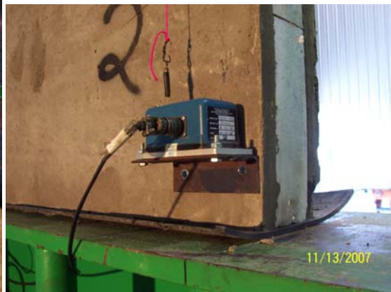
Figures 8A and 9A: Lateral and axial transducer setup (respectively)
