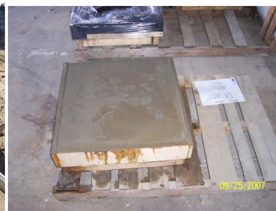
Figures 13 and 14: Smoothing of mortar in wooden form
