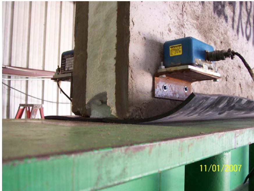
Figure 2A: Axial-compression transducer locations and EPDM rubber installation
