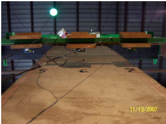
Figures 8A and 9A: Lateral and axial transducer setup (respectively)
