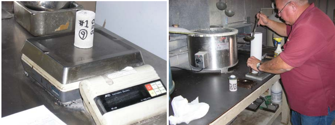
Figures 19 and 20: Labeling, weighing, and sulfur capping of mortar cores
