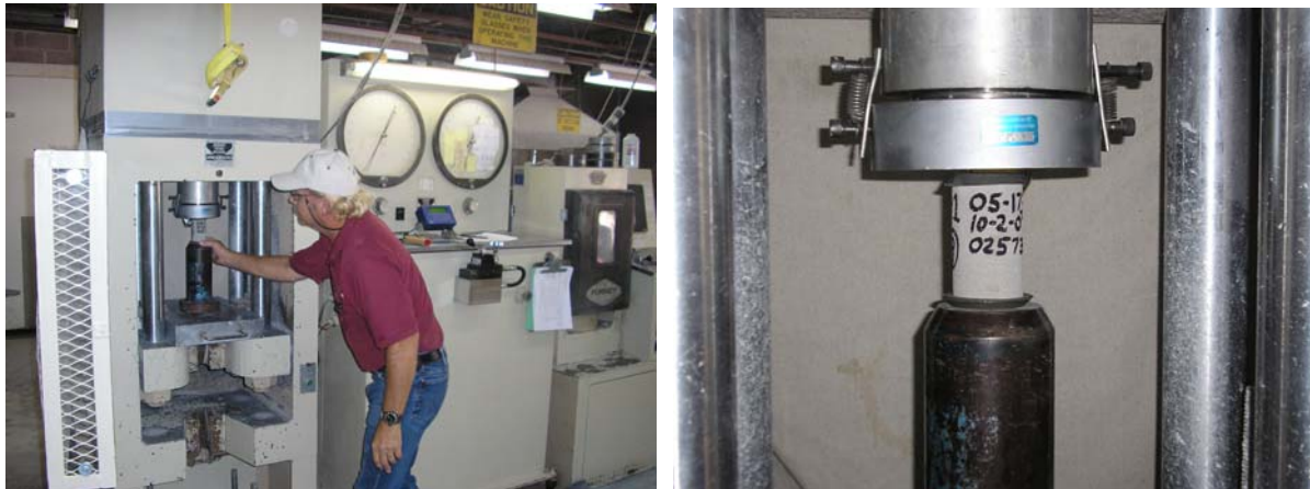
Figures 21 and 22: Cylinder core testing machine and placement of cores into apparatus
