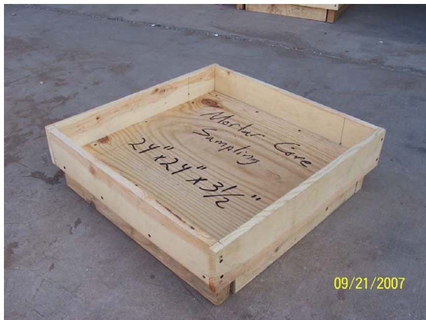
Figure 10: Wooden form for mortar core sampling
