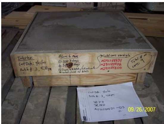
Figures 15 and 16: Mortar form labeling and sealing with plastic sheathing
