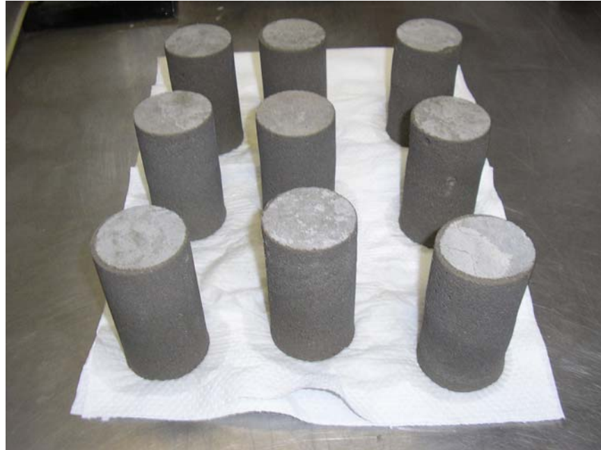
Figure 20: Mortar cores after drilling
