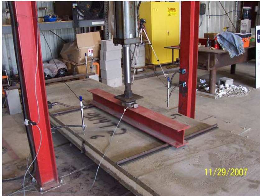
Figure 11: Transverse test setup for 4' x 14' walls (overall view)
