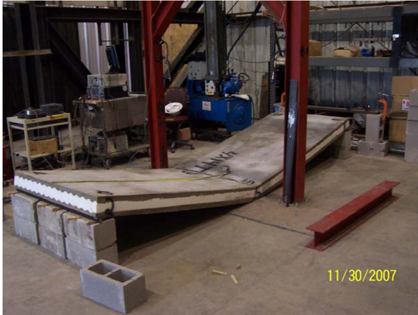
Figure 7A: 4X14T3 Failure mode
