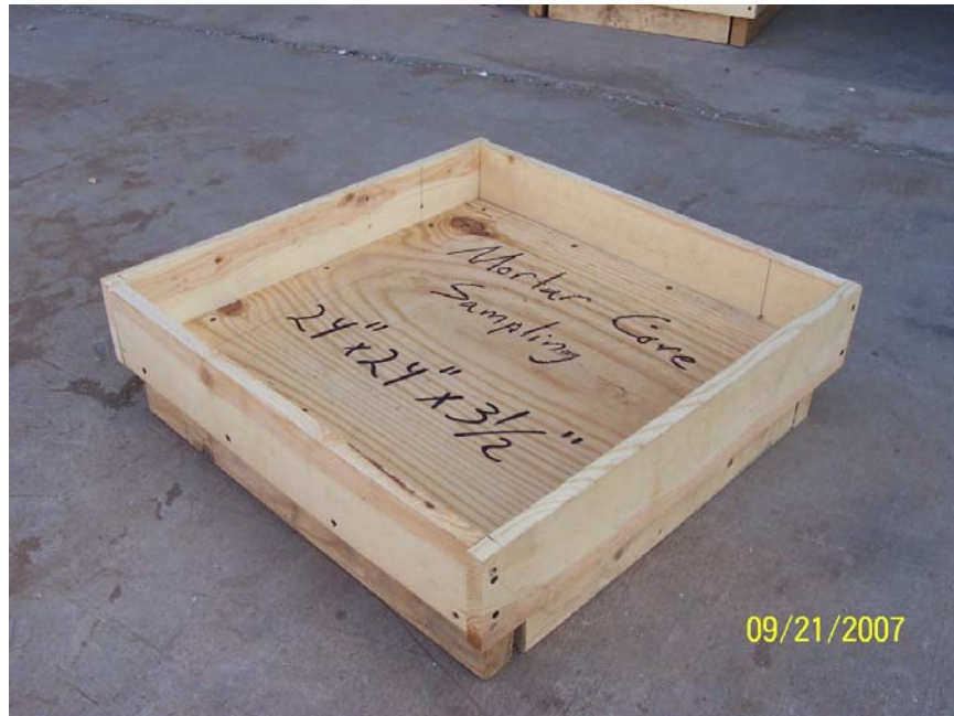
Figure 12: Wooden form for mortar core sampling
