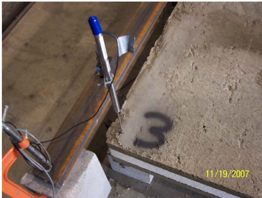
Figure 2A: Transverse-flexural transducer locations
