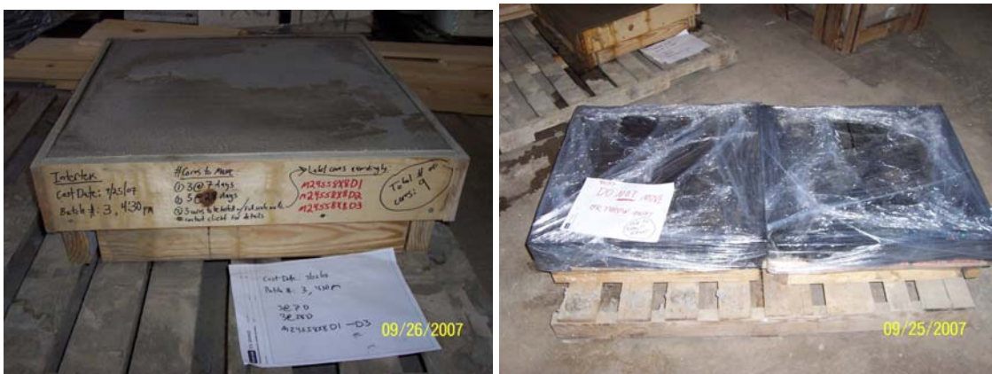
Figures 17 and 18: Mortar form labeling and sealing with plastic sheathing
