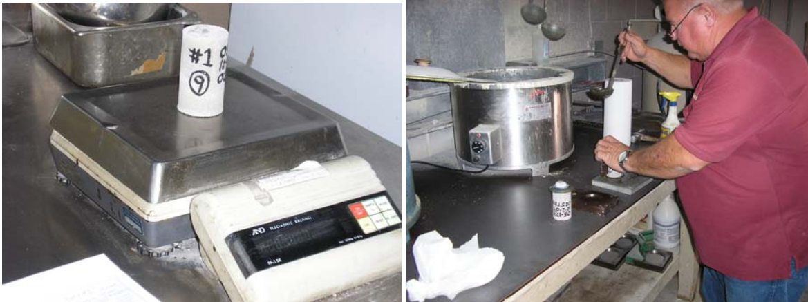
Figures 21 and 22: Labeling, weighing, and sulfur capping of mortar cores
