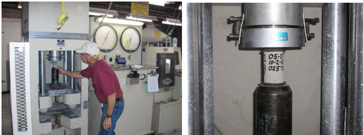
Figures 23 and 24: Cylinder core testing machine and placement of cores into apparatus
