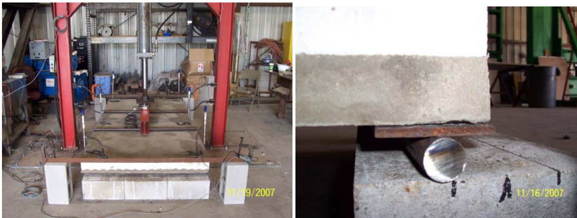
Figures 8 and 9: Flexural Test setup (4' x 8') and 3" wide roller end bearing
