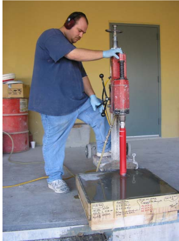
Figure 19: Drilling of mortar cores
