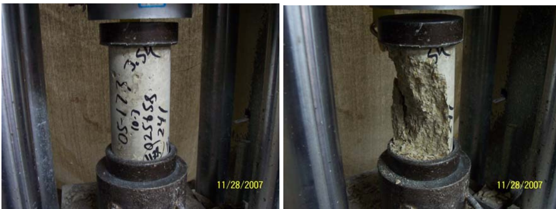
Figures 26 and 27: 4x8 concrete cylinder setup and failure mode
