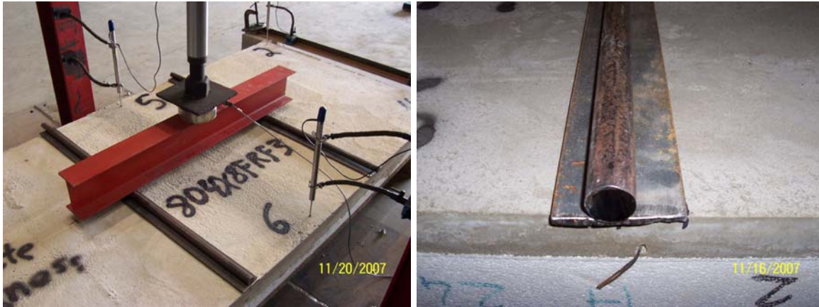
Figures 10 and 11: Third-Point loading setup (top view) and top loading bearing location
