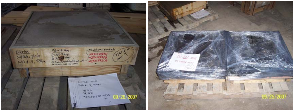
Figures 18 and 19: Mortar form labeling and sealing with plastic sheathing
