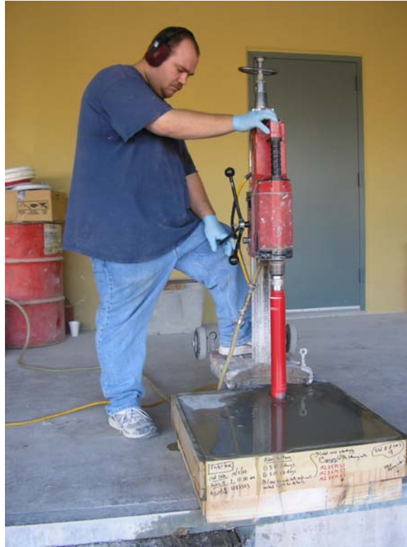
Figure 20: Drilling of mortar cores
