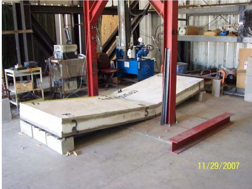
Figure 7A: 150_4X12FRF3 Failure mode
