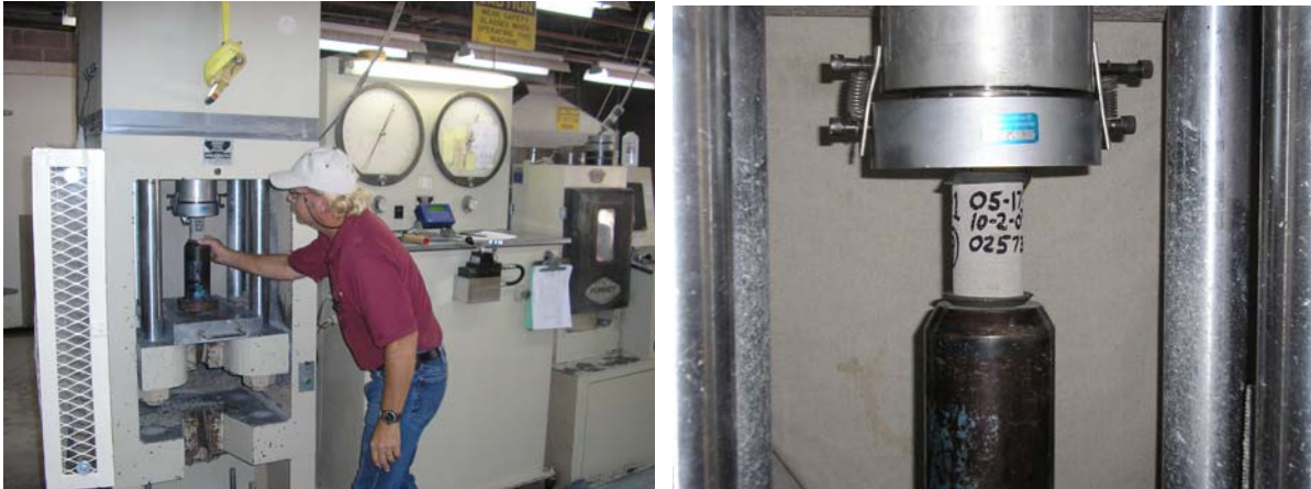
Figures 24 and 25: Cylinder core testing machine and placement of mortar core into apparatus
