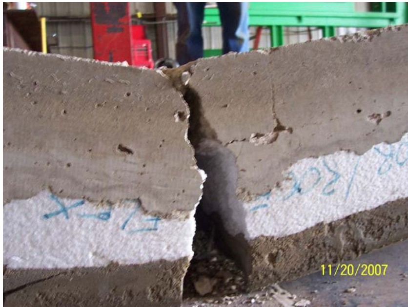
Figure 4A: 80_4X8FRF3 Failure mode (close-up)
