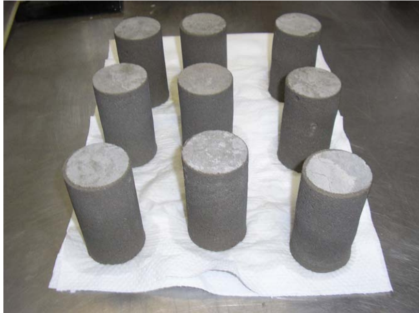
Figure 21: Mortar cores after drilling
