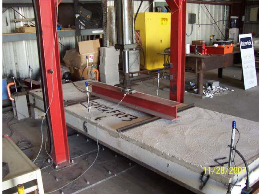
Figure 12: Floor/roof flex test setup for 4' x 12' samples (overall view)
