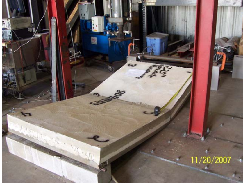
Figure 3A: 80_4X8FRF3 Failure mode
