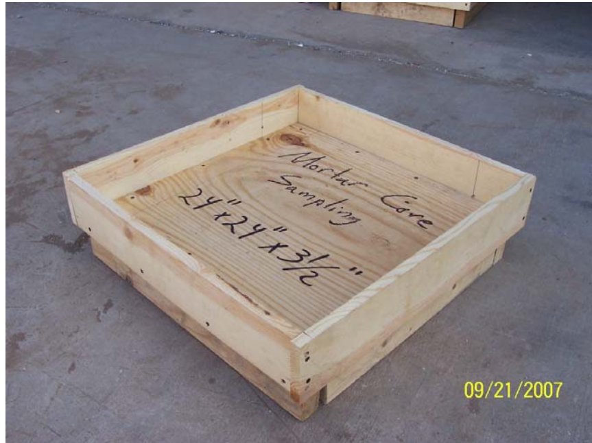
Figure 13: Wooden form for mortar core sampling
