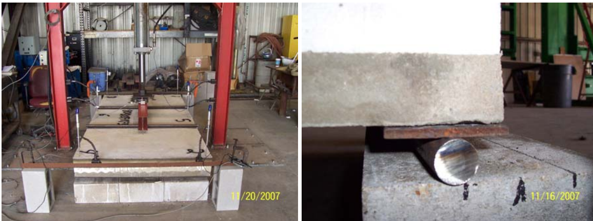
Figures 8 and 9: Floor/roof flexural test setup (4' x 8') and 3" wide roller end bearing
