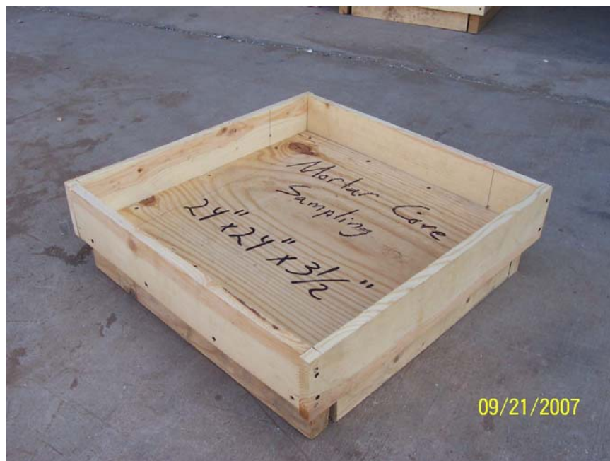
Figure 30: Wooden form for mortar core sampling
