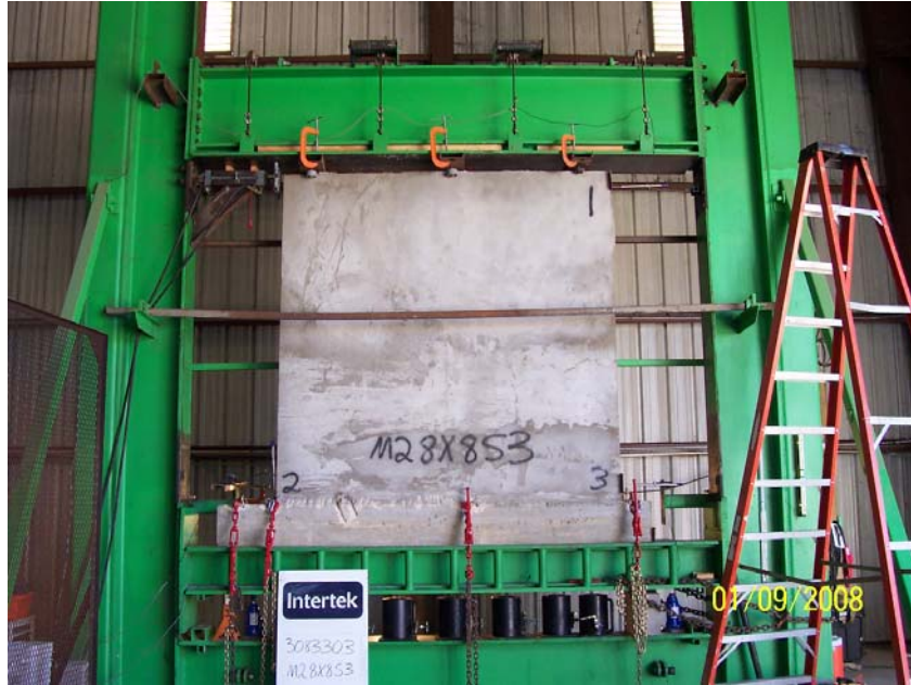
Figure 28: Setup for 8' x 8' shear wall
