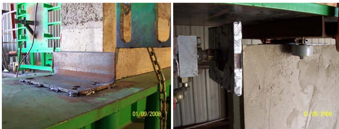
Figures 26 and 27: Stop plate (left) and loading point with rollers (right)
