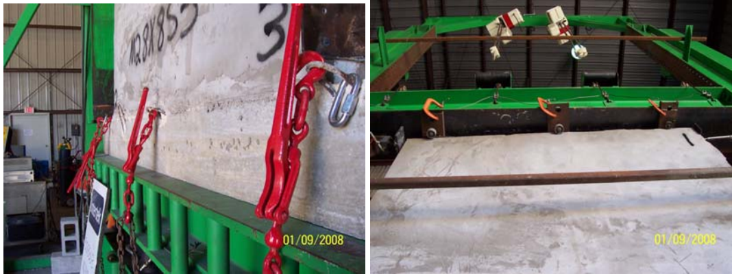
Figures 24 and 25: Boomers holding down footer (left) and lateral guides on wall (right)
