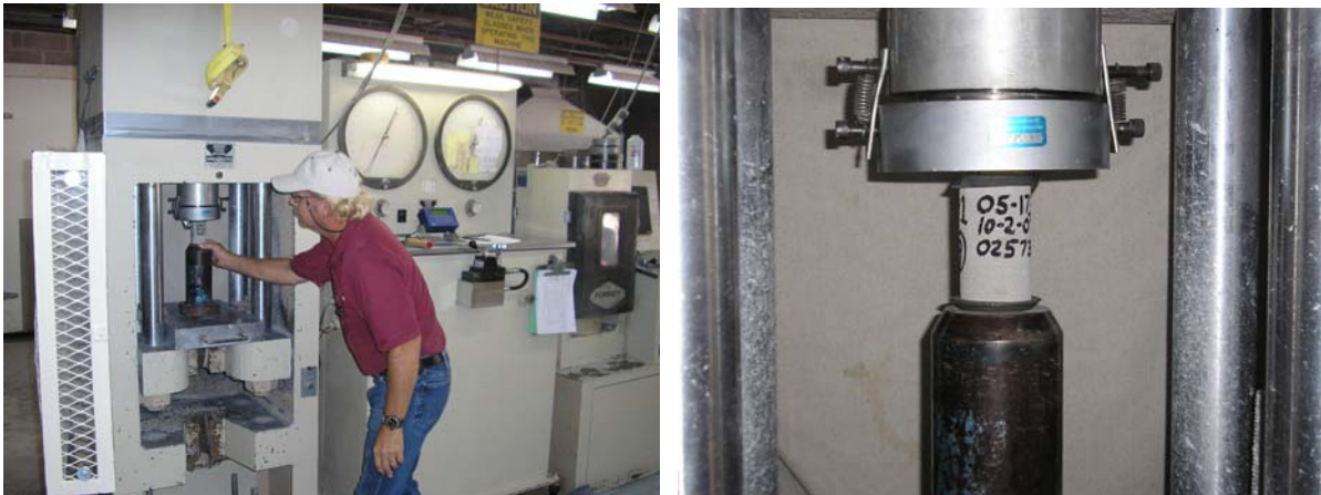
Figures 41 and 42: Cylinder core testing machine and placement of cores into apparatus
