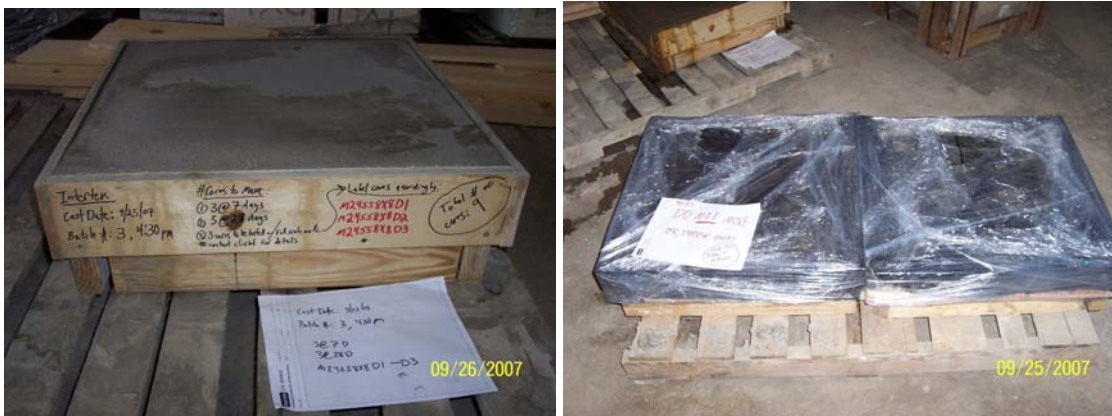
Figures 35 and 36: Mortar form labeling and sealing with plastic sheathing
