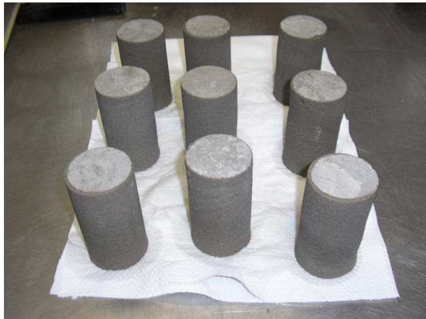
Figure 38: Mortar cores after drilling
