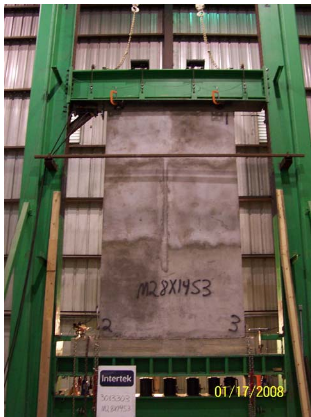
Figure 29: Setup for 8' x 14' shear wall
