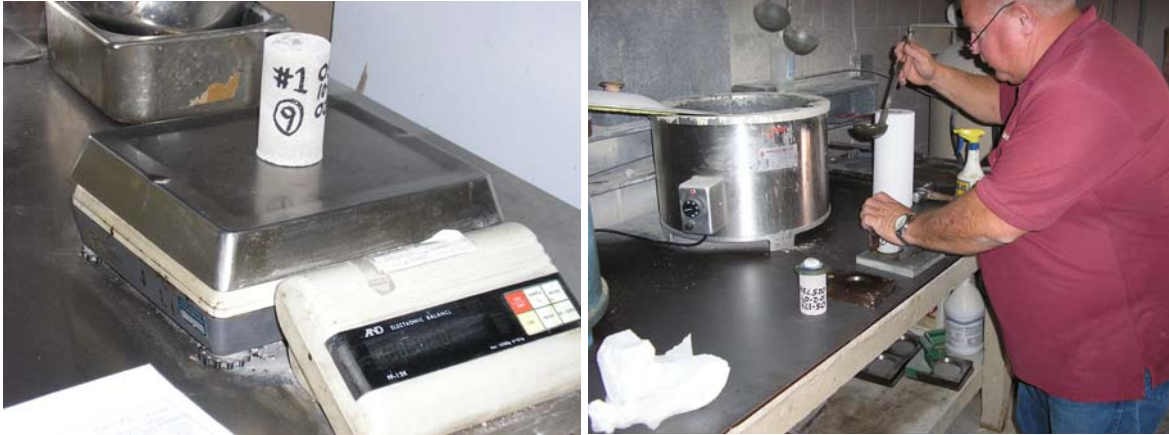
Figures 39 and 40: Labeling, weighing, and sulfur capping of mortar cores
