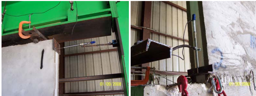
Figures 2A and 3A: LVDT #1 (left) and #2 (right) locations
