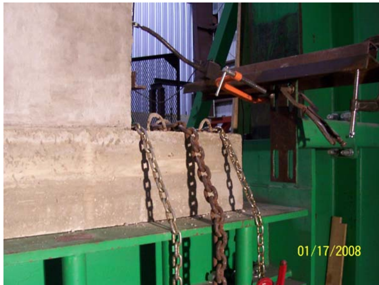
Figures 8A: Rear view of chains and boomsers setup
