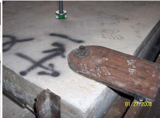
Figures 17 and 18: 3" In-plane steel rollers (left) and top view of hinge connection (right)
