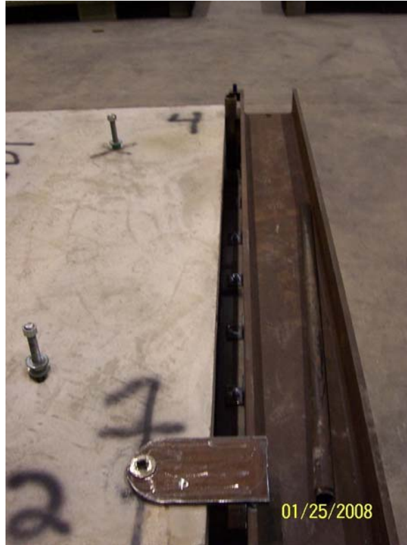
Figure 16: Reaction support with hinge (foreground) and vertical roller (background)
