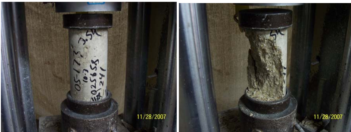
Figures 35 and 36: 4x8 concrete cylinder setup and failure mode
