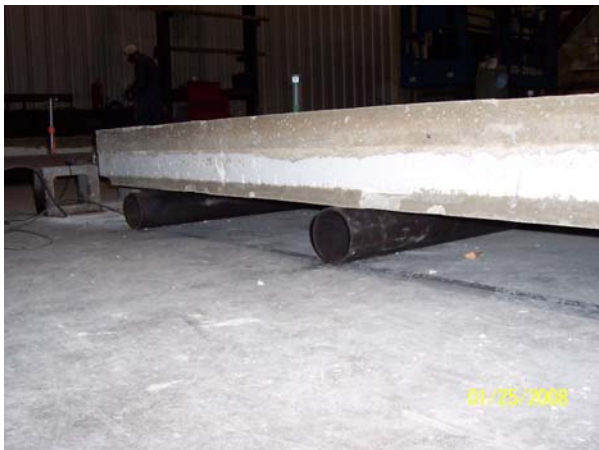
Figures 17 and 18: 3" In-plane steel rollers (left) and top view of hinge connection (right)
