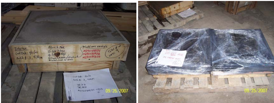
Figures 27 and 28: Mortar form labeling and sealing with plastic sheathing
