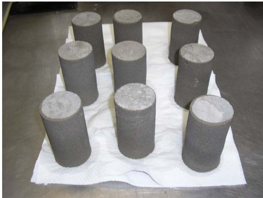
Figure 30: Mortar cores after drilling
