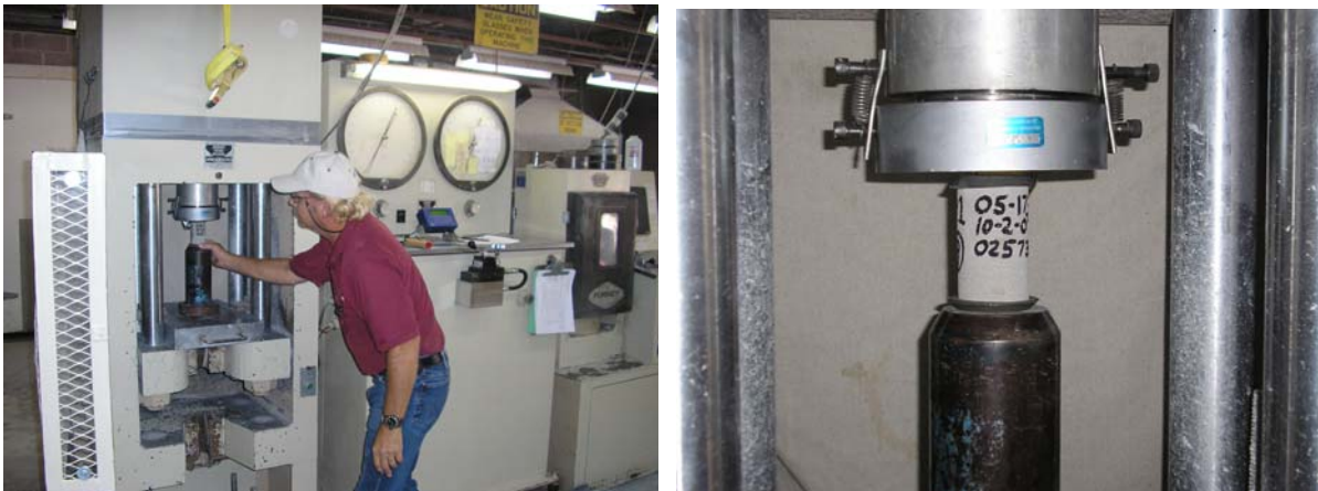
Figures 33 and 34: Cylinder core testing machine and placement of cores into apparatus
