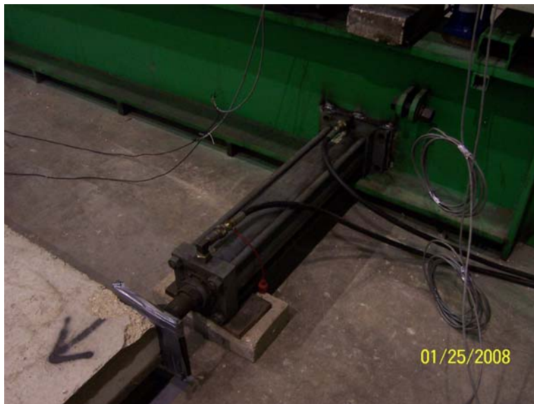
Figure 15: Hydraulic cylinder installation to rigid support beam
