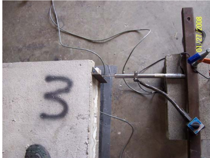
Figure 3A: LVDT #3 location (in-plane with load)
