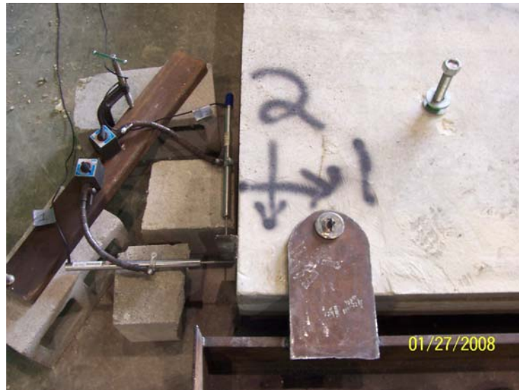
Figure 2A: LVDT #1 (parallel) and #2 (perpendicular) to reaction I-beam
