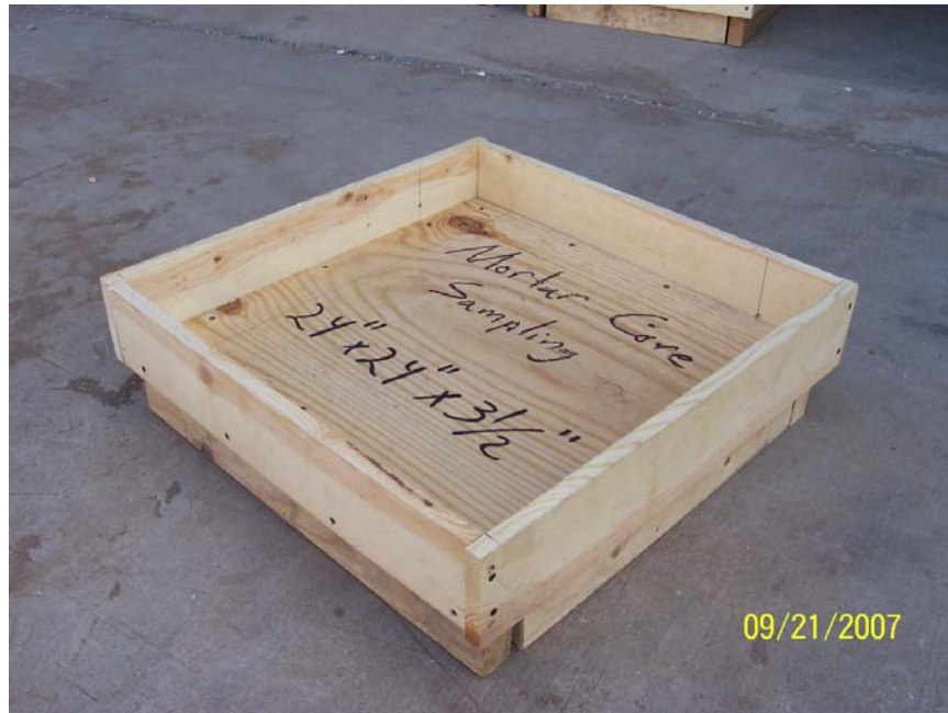
Figure 22: Wooden form for mortar core sampling
