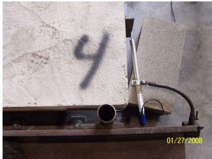
Figure 4A: LVDT #4 location (perpendicular with load)
